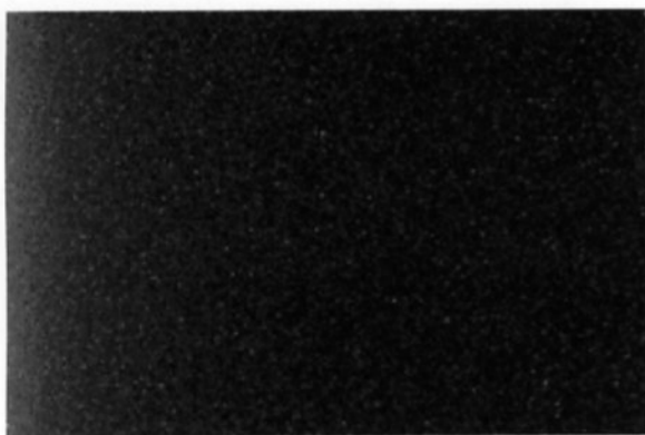
Jim Carlson Dark Frame showing "hot pixels" on the SBIG ST-8XE
